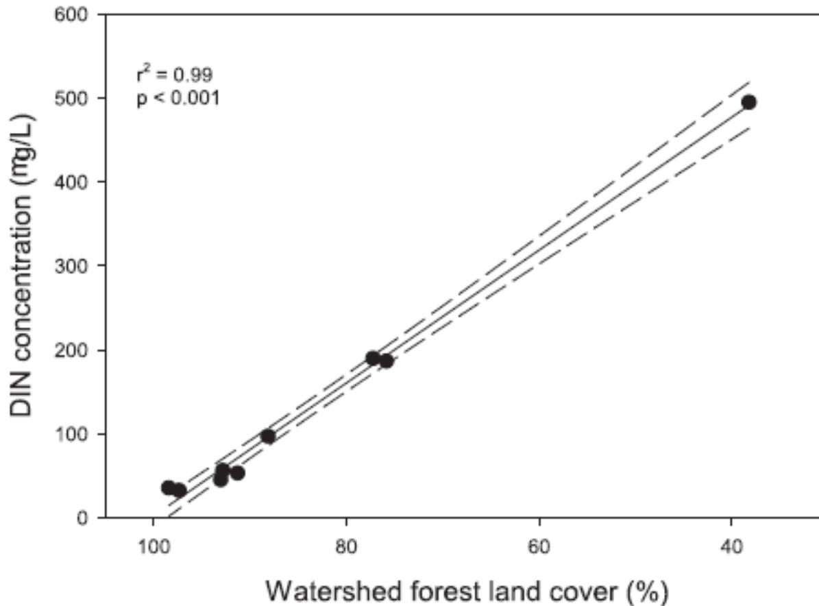
***Figure 7. Stream dissolved inorganic nitrogen (DIN) concentrations across a gradient of forest cover. Basin forest cover explains 99% of the variation in stream DIN. Source: Adapted with permission from Webster and colleagues (2019).***
